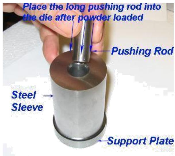
4. Place the long pushing rod into the die with the powder loaded.
