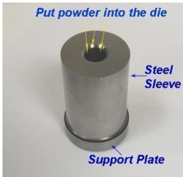
2. Place the sleeve with the rod on the support plate.
