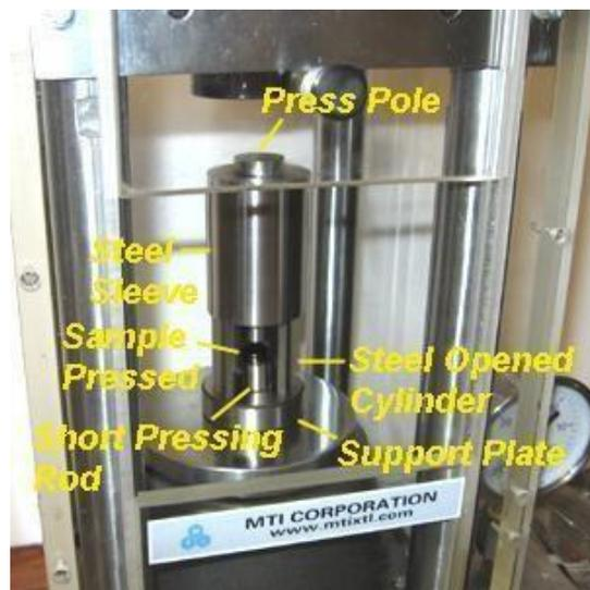
12. Gently push the pressing pole by the lead screw (spinning screw) to get the product.
