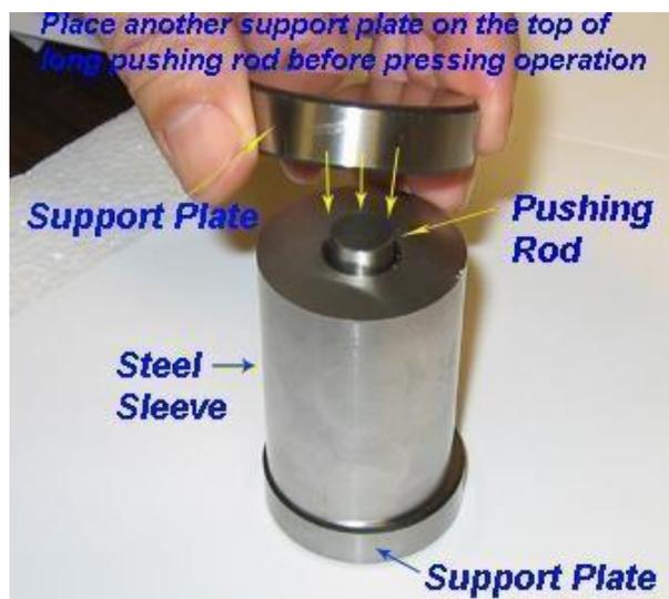
5. Put another support plate on the top of long pushing rod. Die assembling is complete.
