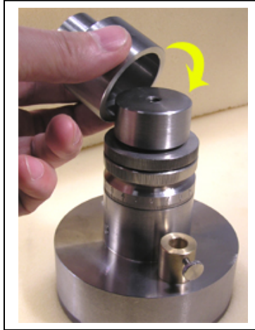
Fig. 17 putting the second force weight back
