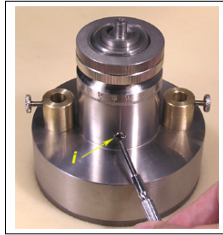
Fig. 5 Loose setting screw (part i) which lock the rod (part j)
