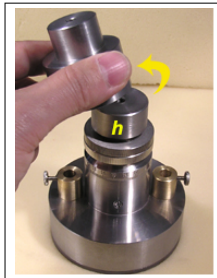
Fig. 3 Take off the second force weight (part b) from central rod locking nut (part h)
