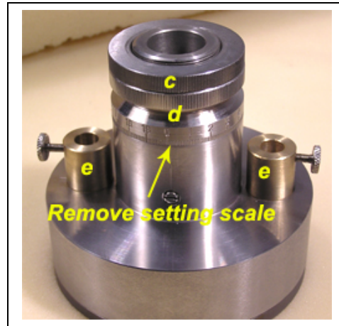
Fig. 9 Remove setting scale on micrometer dials screw (part d)
