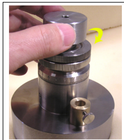
Fig. 16 screwing up the Rod locking nut
