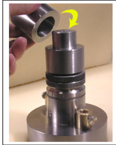
Fig. 18 putting the first force weight back
