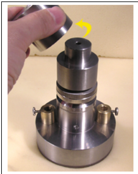
Fig. 2 Take off the first force weight (part a) from the second force weight (part b)
