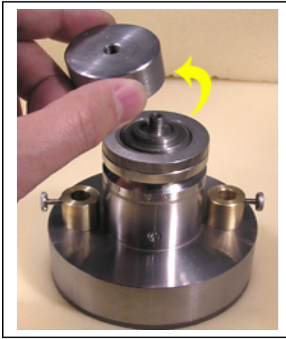
Fig. 4 Remove locking rod assembly (part h)
