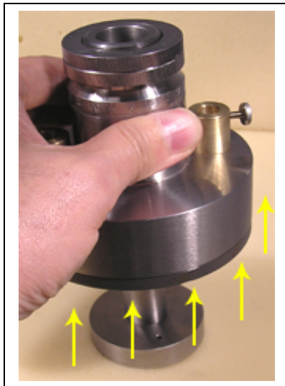
Fig. 6 Lift up the housing straightly
