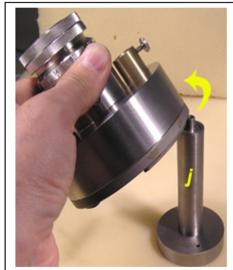
Fig. 7 Take off the housing from the rod (part j)
