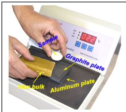
Fig.2 gluing a piece of sample by melting wax on the heating plate
