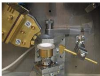
Fig. 4: Please keep the reference sample ( Alumina ) in flat position on the sample holder
