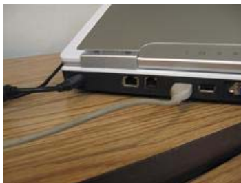
Fig2. (Must plug USB connector into socket on the back of Laptop )
