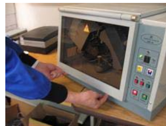
Fig. 3. Please push two buttons on the bottom to open the door
