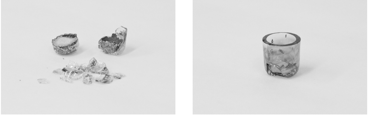
Figure 2.7: Broken quartz crucibles
