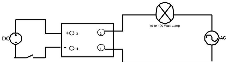
When this is connected, the battery should control when the light is on or off. Applying the 9 volts DC will turn the light on and when you remove the DC voltage, the light bulb should turn-off.
