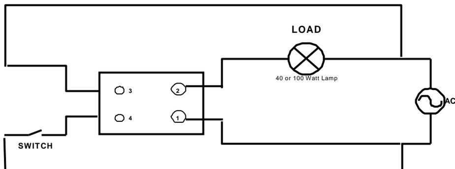
When the switch is open, the light should be off, and with the switch closed, the light should be on. Anything else will indicate a faulty relay.
