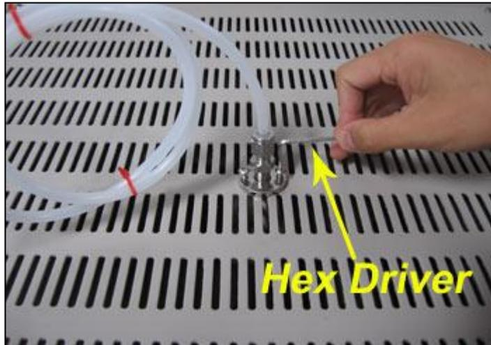
4. To install the tube labeled “inlet” to the inlet, repeat the steps 1-3.
