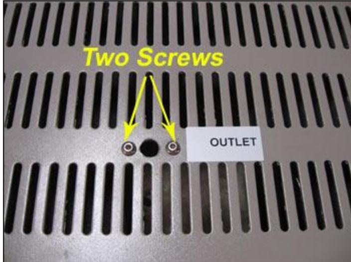
2. Put the **Al<sub>2</sub>O<sub>3</sub> Tube** labeled "outlet" with the flange and gas hose together into the outlet.
