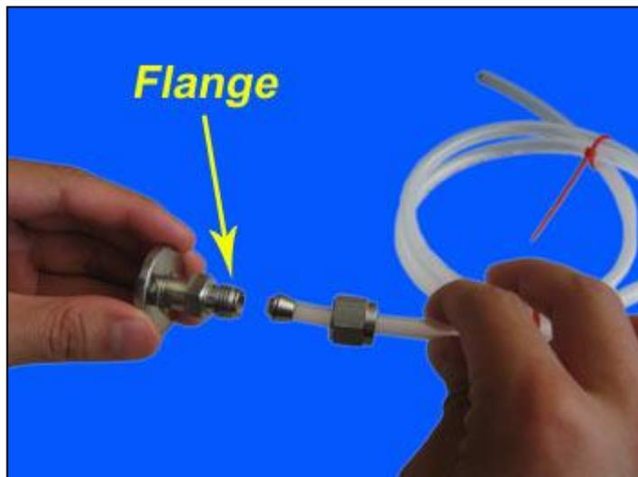
4. Screw the flange cap to flange and make sure it is tight enough.
