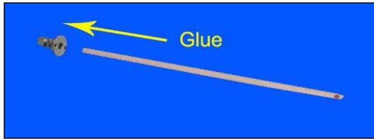
Note: The customer is advised not to change the  $\text{Al}_2\text{O}_3$  tube sticking to the flange.
