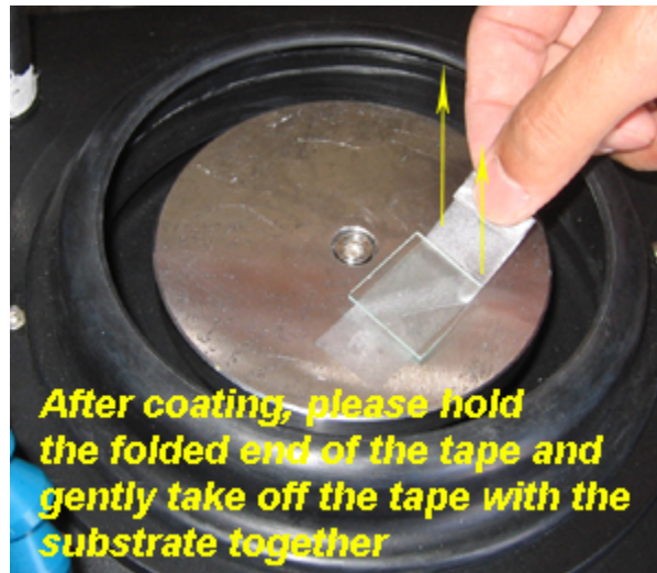
Figure 3, Take off the tape and the substrate together gently by holding the folded end of the tape
